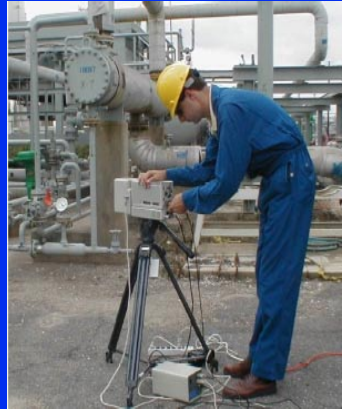
IMSS on Radiance 1 Infrared Camera in Oil Refinery (Precursor to PAT Sherlock Camera)
