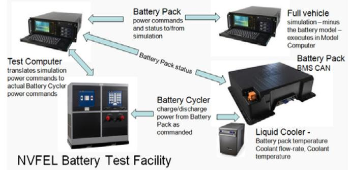
Figure 9. Battery Test Setup at EPA NVFEL Battery Test Facility
