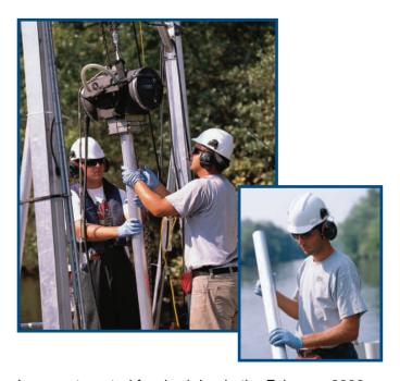
In areas targeted for dredging in the February 2002 ROD, sample locations were identified based on an 80-foot triangular grid. In other areas, a 160-foot triangular grid was used. Sampling locations were transmitted electronically to the sampling vessels and downloaded into each vessel's on-board GPS for accurate positioning. Shore-based control points were established at each Champlain Canal Lock to guide the vessels to pre-programmed coordinates.
