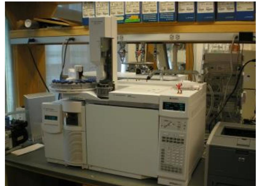
Gas Chromatograph Mass Spectrometer (GC/MS)
