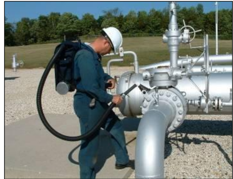
Leak Measurement Using High Volume Sampler
