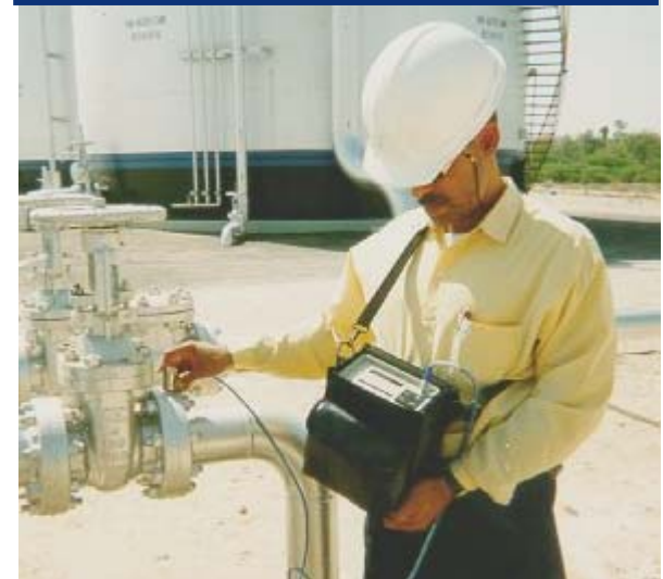
Acoustic Leak Detection
