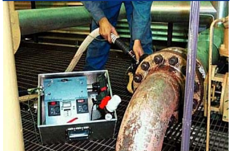
Leak Measurement Using a High Volume Sampler
