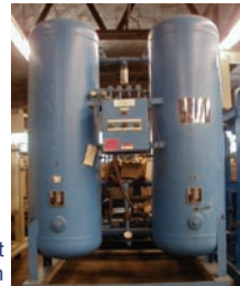
Desiccant Dehydrator Unit Source: usedcompressors.com
