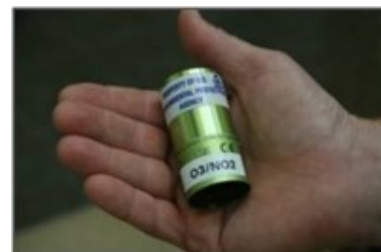
The CairClip air sensor fits in the palm of a hand and collects data on ozone and nitrogen dioxide in the air.
