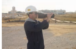
Infrared Leak Detection
