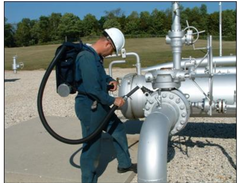
Leak Measurement Using High Volume Sampler
