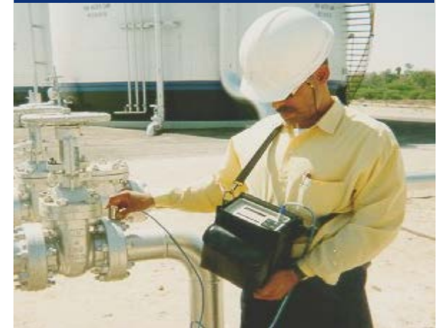
Acoustic Leak Detection
