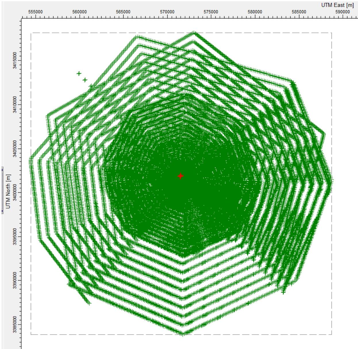
**Figure 12: Near-field Receptor Grid for the Ville Platte Plant Area. The green “+” symbols represent the locations of receptors around the Cabot Ville Platte facility with the location of the maximum design value indicated by the red circle. Some receptors are evident within the facility fenceline itself (red boundary) and were included in the design value calculation using the modeled results.**
