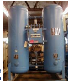
Desiccant Dehydrator Unit Source: usedcompressors.com
