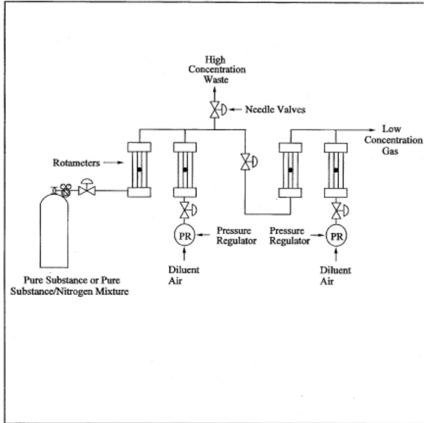
Figure 18-6. Two-Stage Dilution Apparatus.
