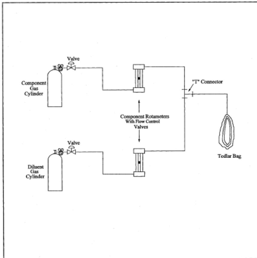
Figure 18-5. Single-Stage Calibration Gas Dilution System.
