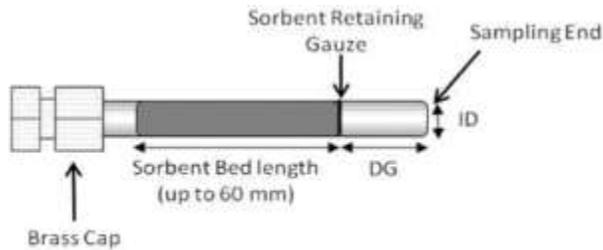
**Figure 6.1. Cross Section View of Passive Sorbent Tube**
