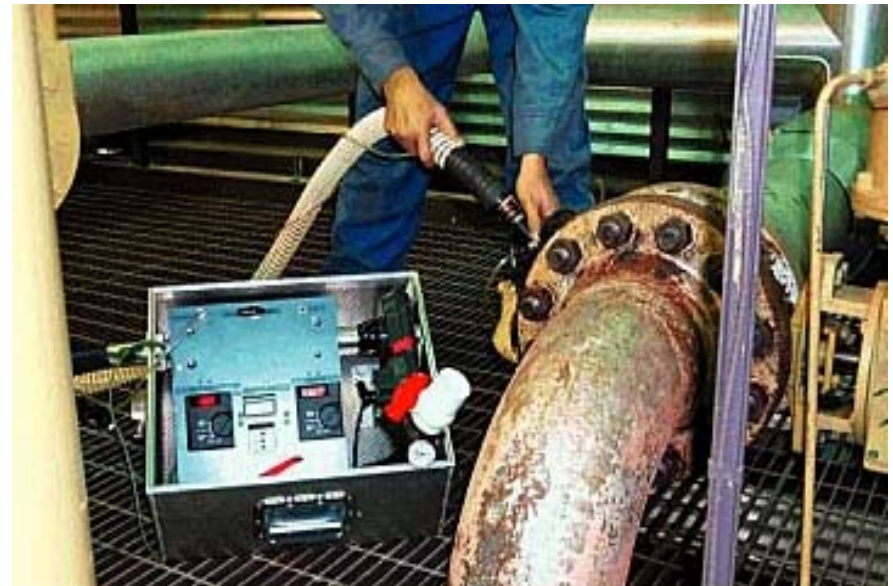
Leak Measurement Using a High Volume Sampler
