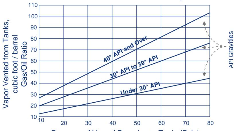
Pressure of Vessel Dumping to Tank (Psig)
