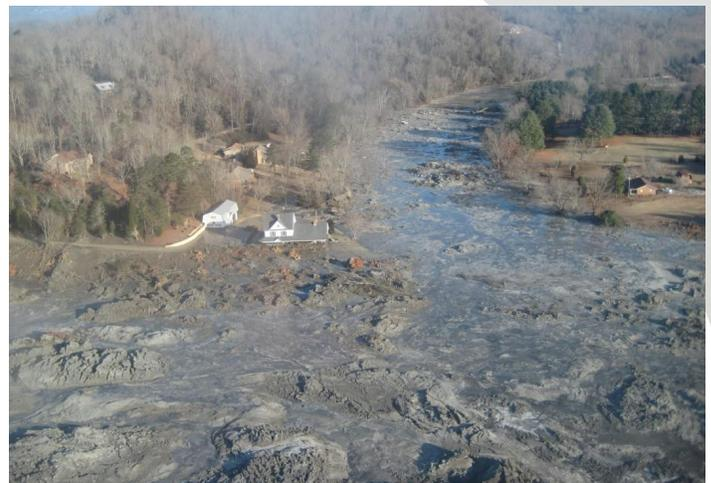
Figure 3. Remaining ash in cell where the breach occurred in 2008 (left). Flow of ash into the Emory River from the breach (right). (Source: EPA)
