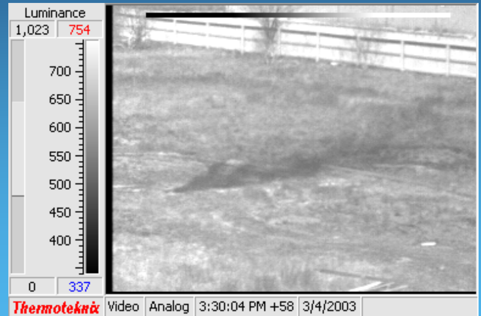
Buried Pipeline Leak
