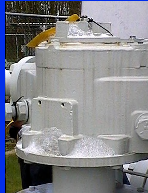
Bubble test on leaking valve
