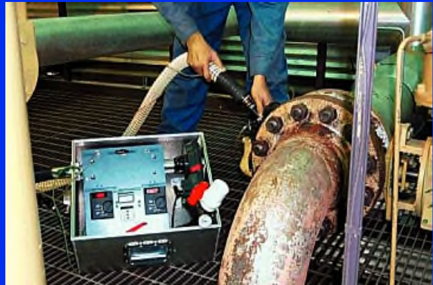
Leak Measurement Using a High Volume Sampler
