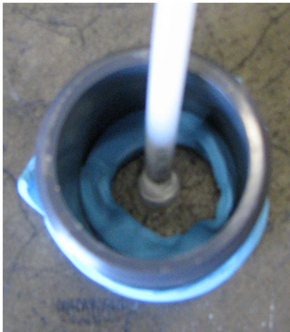
Figure 3. Water dam above slab, temporarily sealed to the floor with Sticky-Tac™
