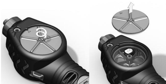
Ensure that the sensor seal (9), on the inside of the sensor cover is not disturbed.
