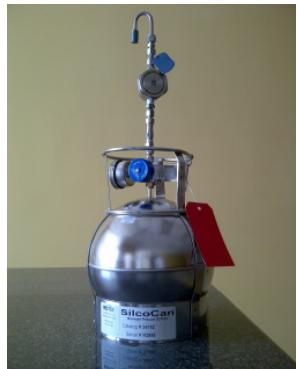
With the property owner / occupant's permission, samples of air from a crawlspace, basement, garage and/or living space are collected in basket-ball sized steel canisters (called Summa Canisters) that sample the air over a specified period of time (usually 8 hours in commercial settings and 24-hours in residential settings). Afterwards, the air is sent to a certified laboratory and analyzed for volatile organic compounds (VOC).
