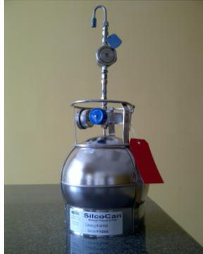
With the property owner / occupant's permission, samples of air from a crawlspace, basement, garage and/or living space are collected in basket-ball sized steel canisters (called Summa Canisters) that sample the air over a specified period of time (usually 8 hours in commercial settings and 24-hours in residential settings). Afterwards, the air is sent to a certified laboratory and analyzed for volatile organic compounds (VOC).
