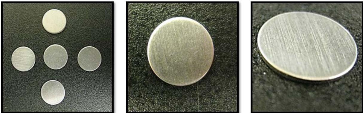
Fig. 1: Examples of typical acceptable 430 SS carriers.
