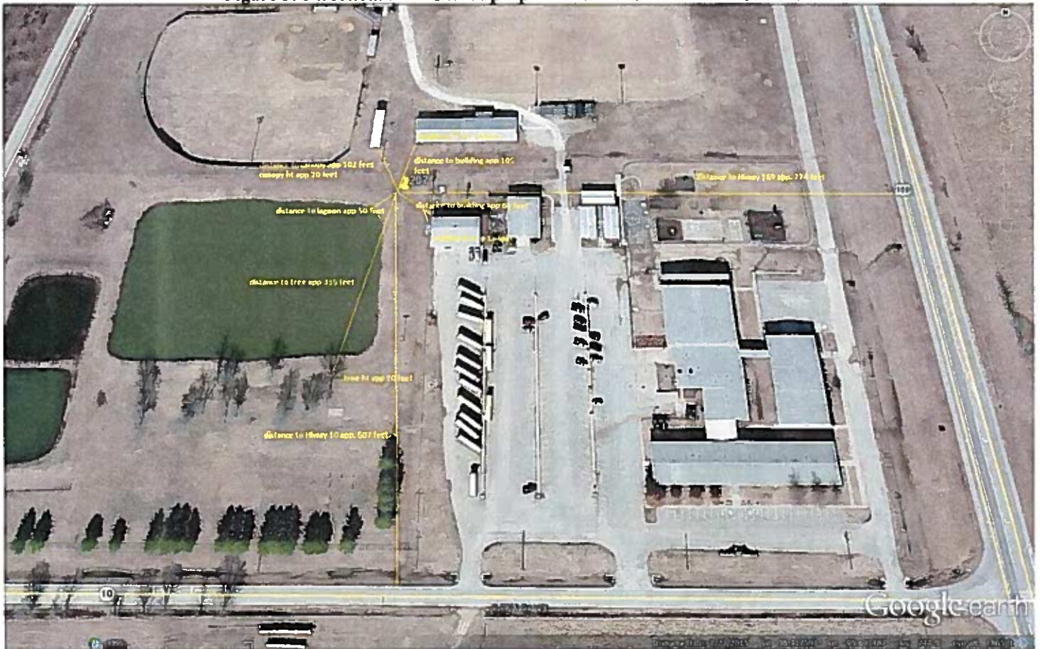
Figure 4: Distance of proposed site location from nearby roads, vegetation, buildings, and other possible obstructions and sources.
