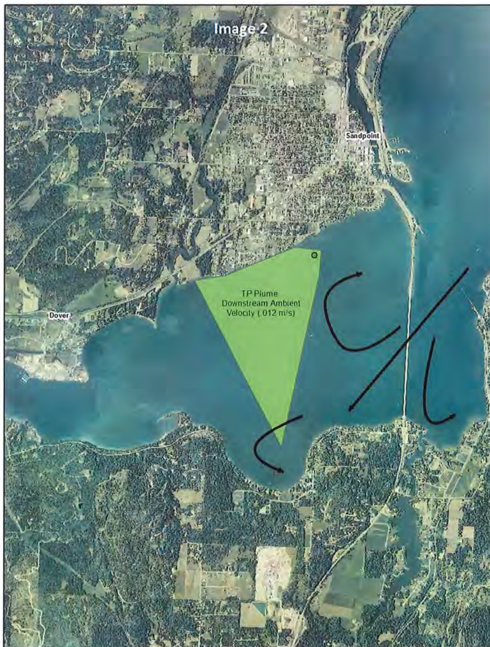
Image 2 Early CORMIX Modeling Scenario Phosphorus Concentration of 2867 \mu g/L; Facility Design Flow of 3.62mgd and River Flow of 8,448cfs
