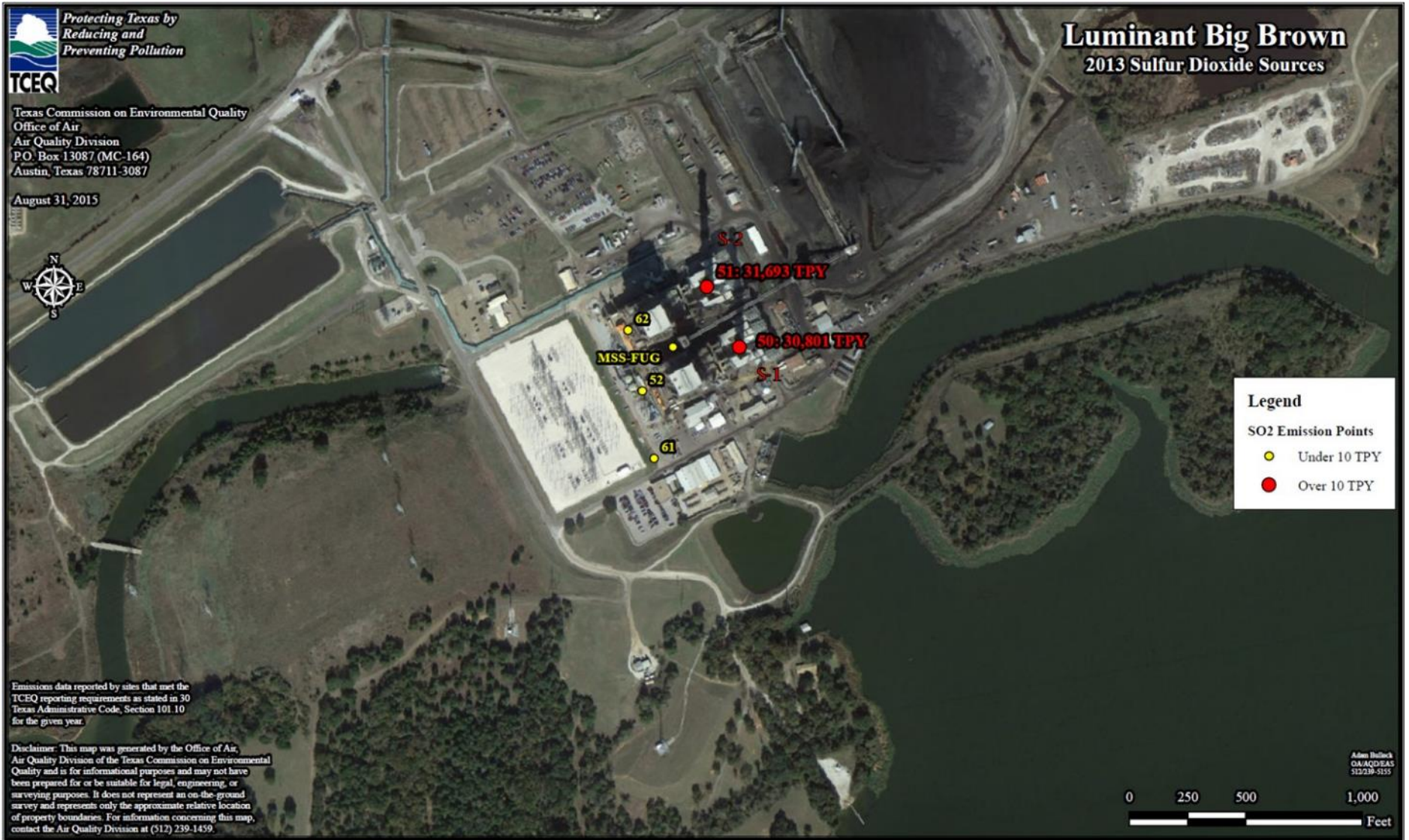
Figure 2: Big Brown Sulfur Dioxide (SO 2 ) Stacks and Emissions for 2013
