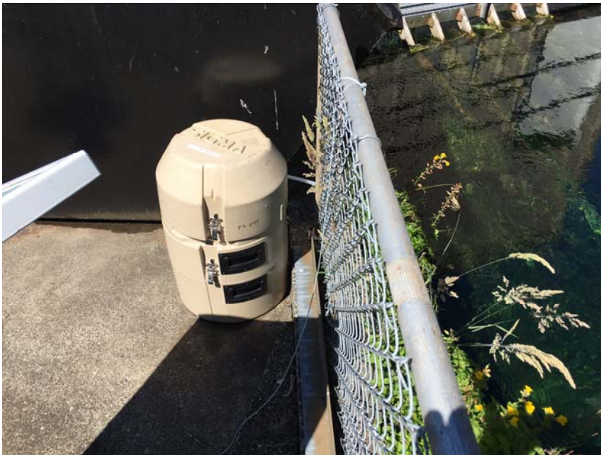
8- Automatic sampler deployed at CNFH influent location
