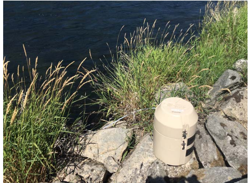
16- Automatic sampler deployed at DNFH downstream location
