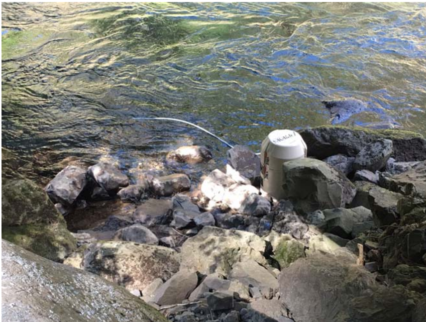
3- Automatic sampler deployed at LWSNFH downstream
