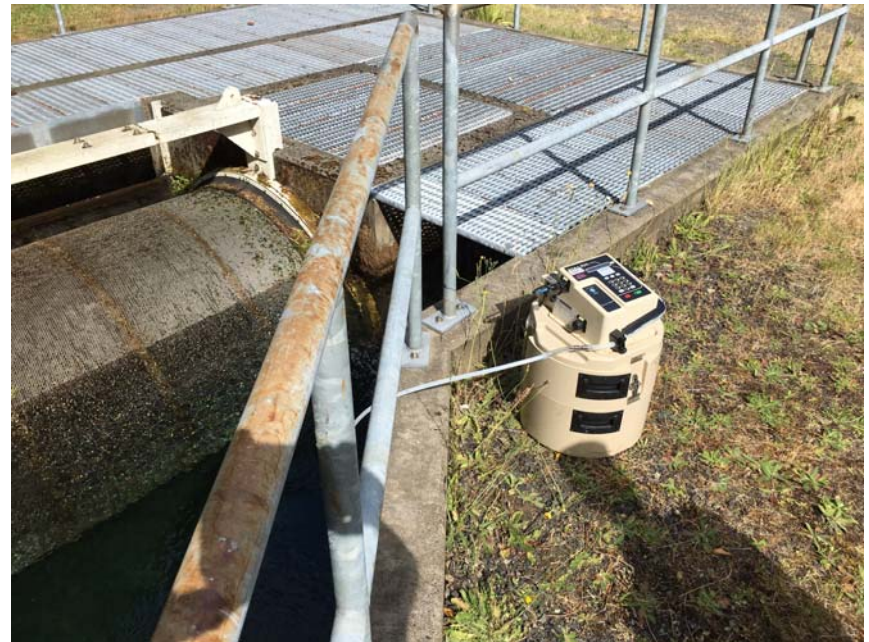
2 – Automatic sampler deployed at LWSNFH influent location
