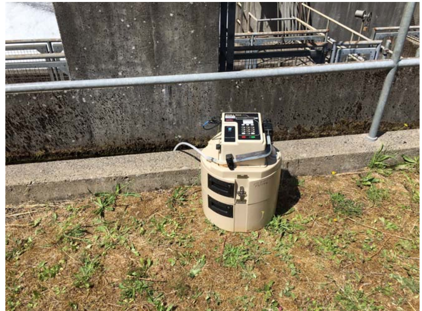
4- Automatic sampler deployed at LWSNFH outfall
