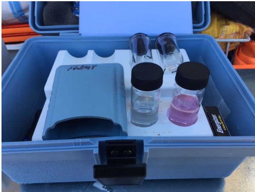
19- Chlorine test kit – effluent location
