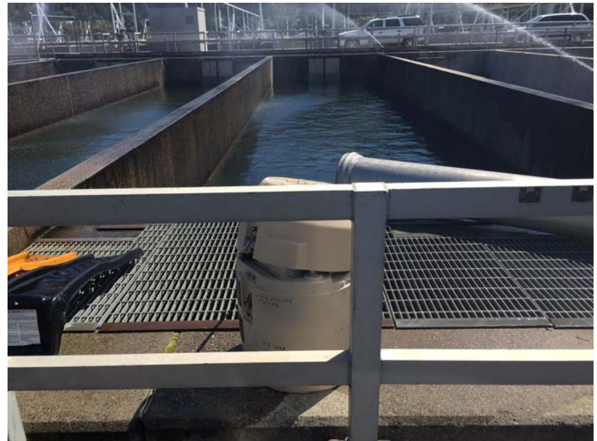
14- Automatic sampler deployed at CDNFH effluent location
