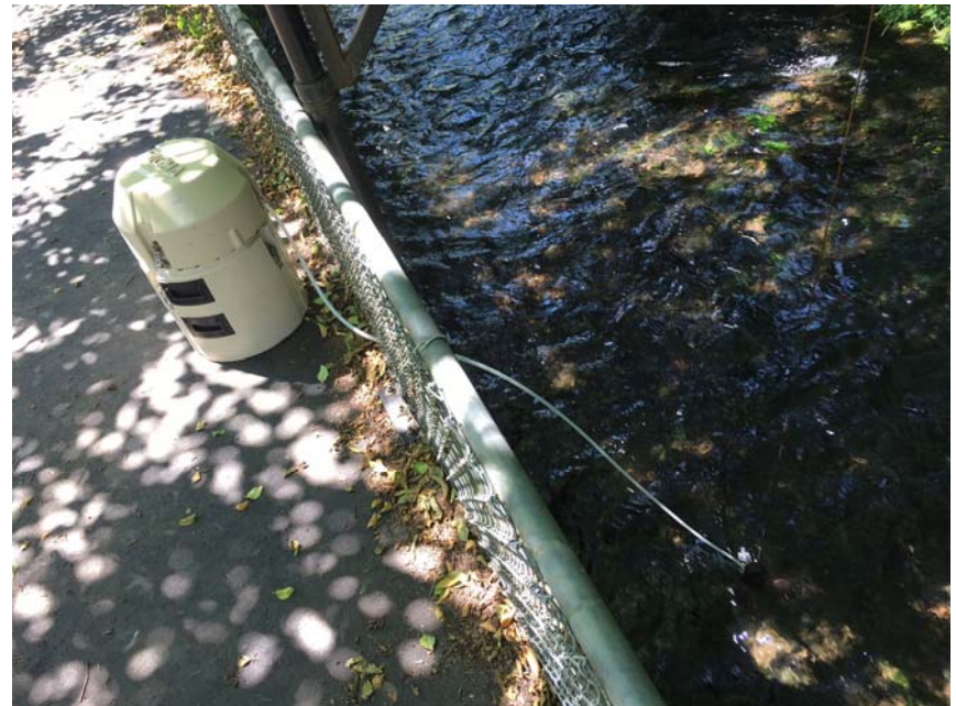
9- Automatic sampler deployed at CNFH outfall location
