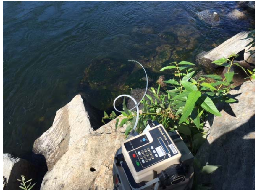
20- Automatic sampler deployed at CIWFH downstream location
