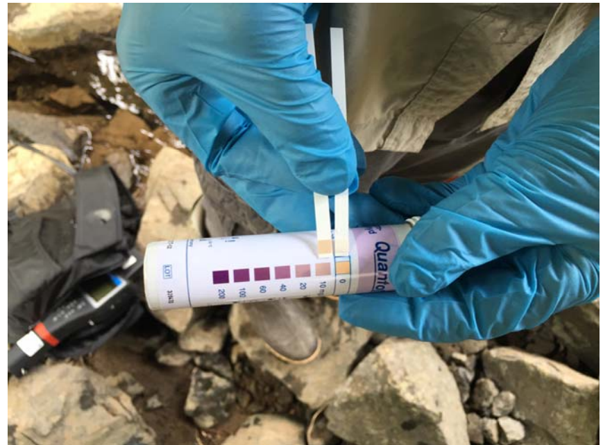
6 – Screening for formaldehyde with test kit downstream
