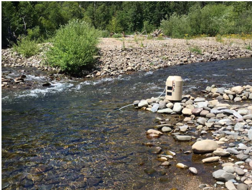
10- Automatic sampler deployed at CNFH downstream location
