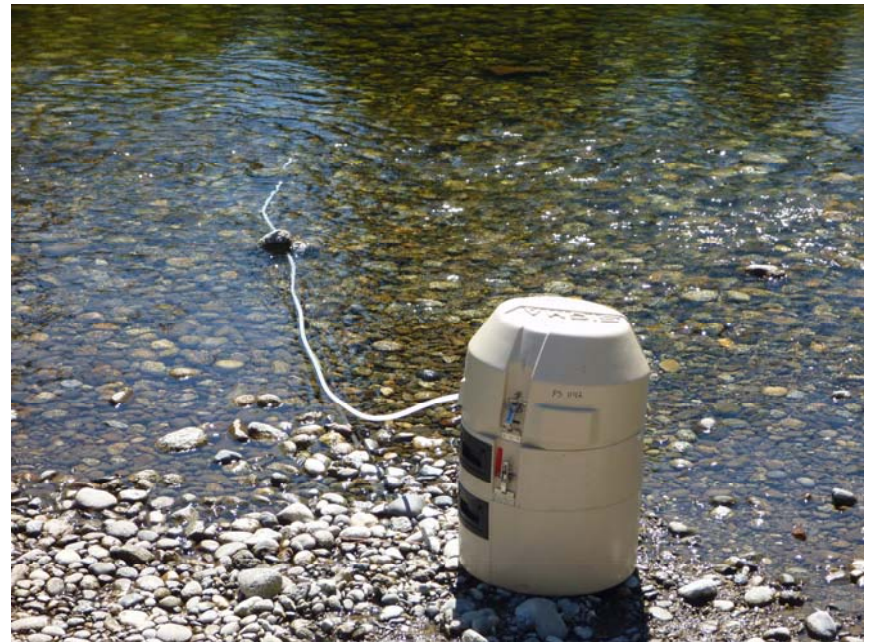
24- Automatic sampler deployed at LNFH downstream location
