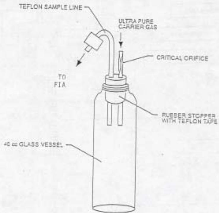
Figure 2. VOC sampling vessel.
