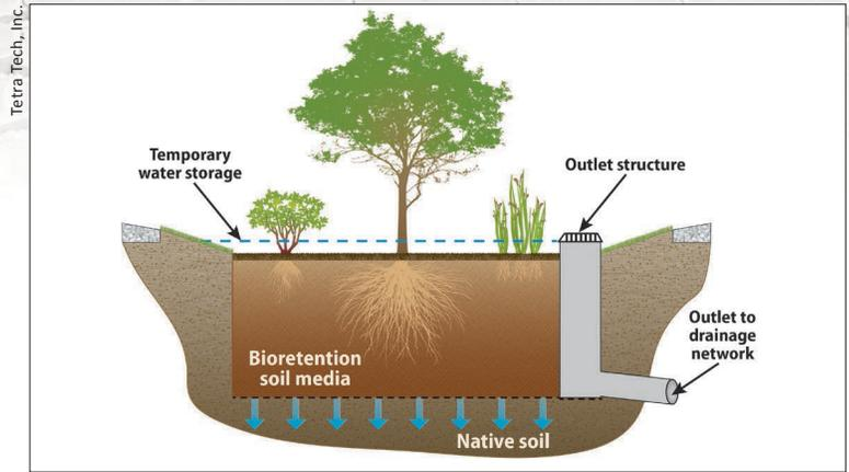
Figure 4. Overflow drain. Stormwater fills the practice and begins soaking through the bioretention soil media and into native soil. Excess water can spill through an outlet structure to an alternative drainage network.
