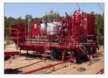
Example of Green Completion Equipment (Source: Weatherford)
