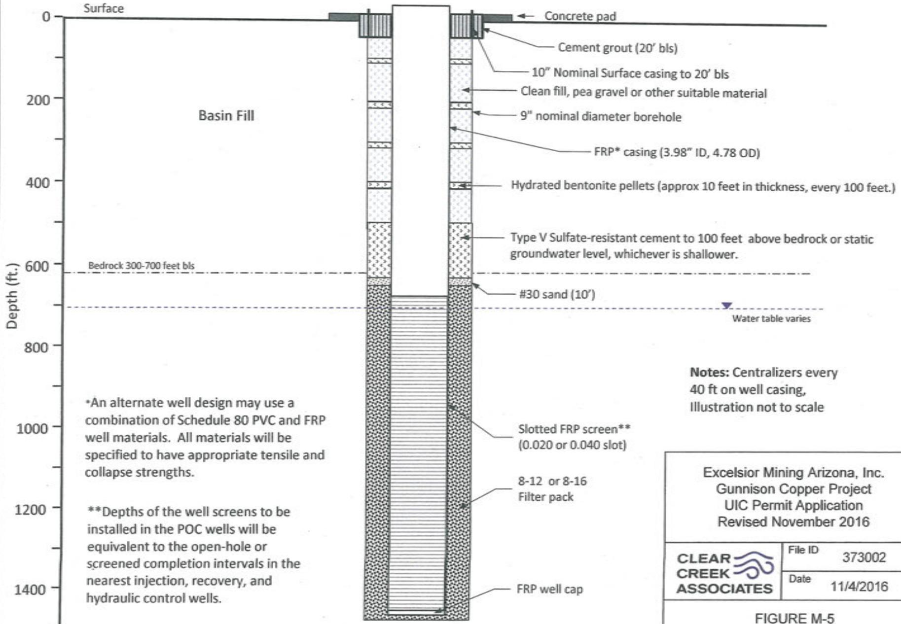
\*An alternate well design may use a combination of Schedule 80 PVC and FRP well materials. All materials will be specified to have appropriate tensile and collapse strengths.
