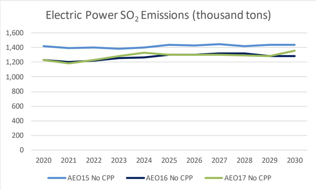
**Figure 7-9. Electric Power Sector SO<sub>2</sub> Emissions in Annual Energy Outlook Projections without the CPP (thousand short tons)**
