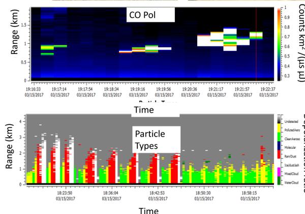
Figure 3. The Relative plume height is interpreted from the MiniMPL backscatter (on March 15). The range indicates distance from Lidar to particle. (Top) particle counts, the lighter the color the higher the intensity of backscatter, with white being off scale. (Bottom) depolarization ratio, used to determine particle types. Smoke is indicated by yellow and red; white is underdetermined by the software.
