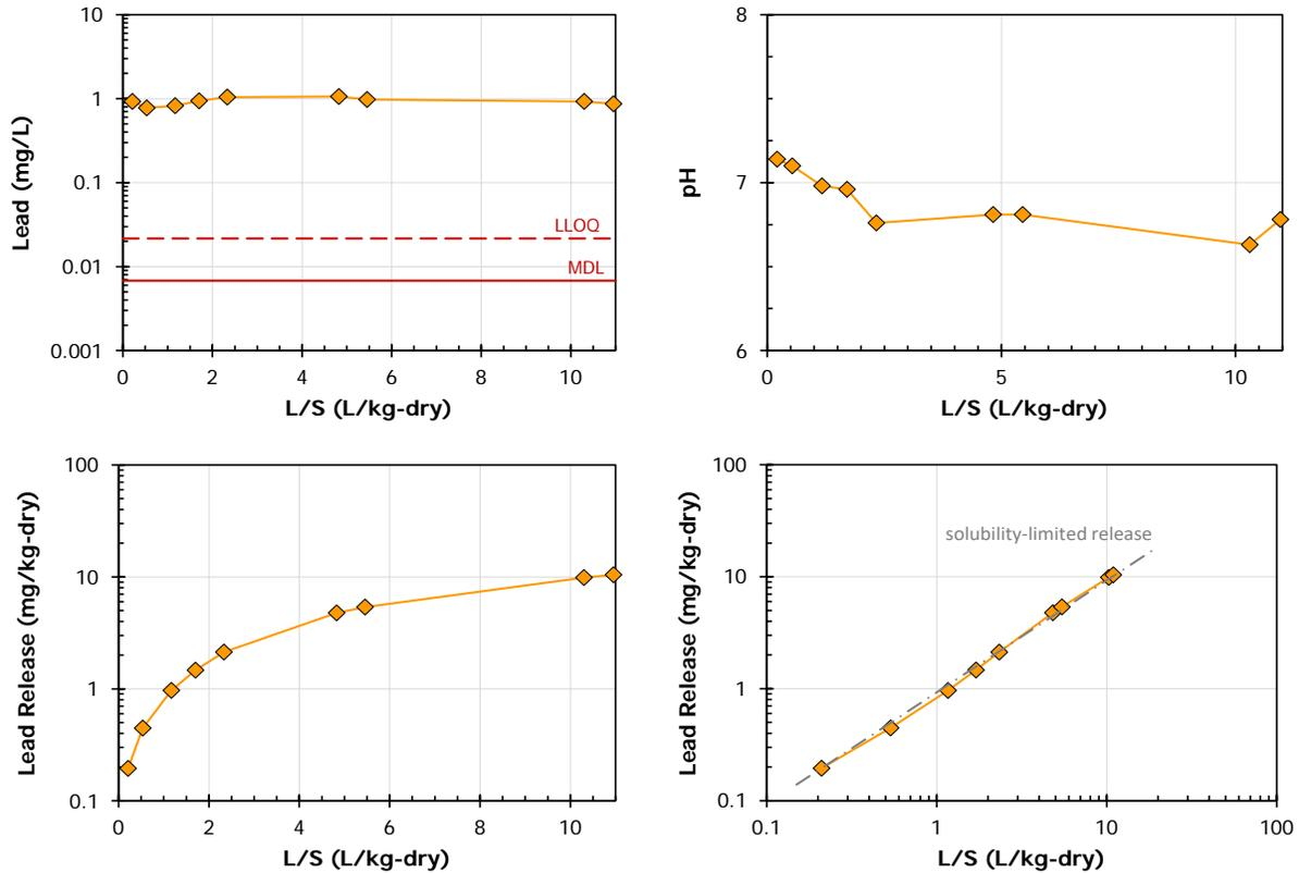
**Figure 3-4. Example results from Method 1314 for lead as a function of L/S from a contaminated smelter site soil (CFS):** Concentration (top, left), eluate pH (top, right) and cumulative release on Cartesian axis (lower, left) and logarithmic axis (lower, right).
