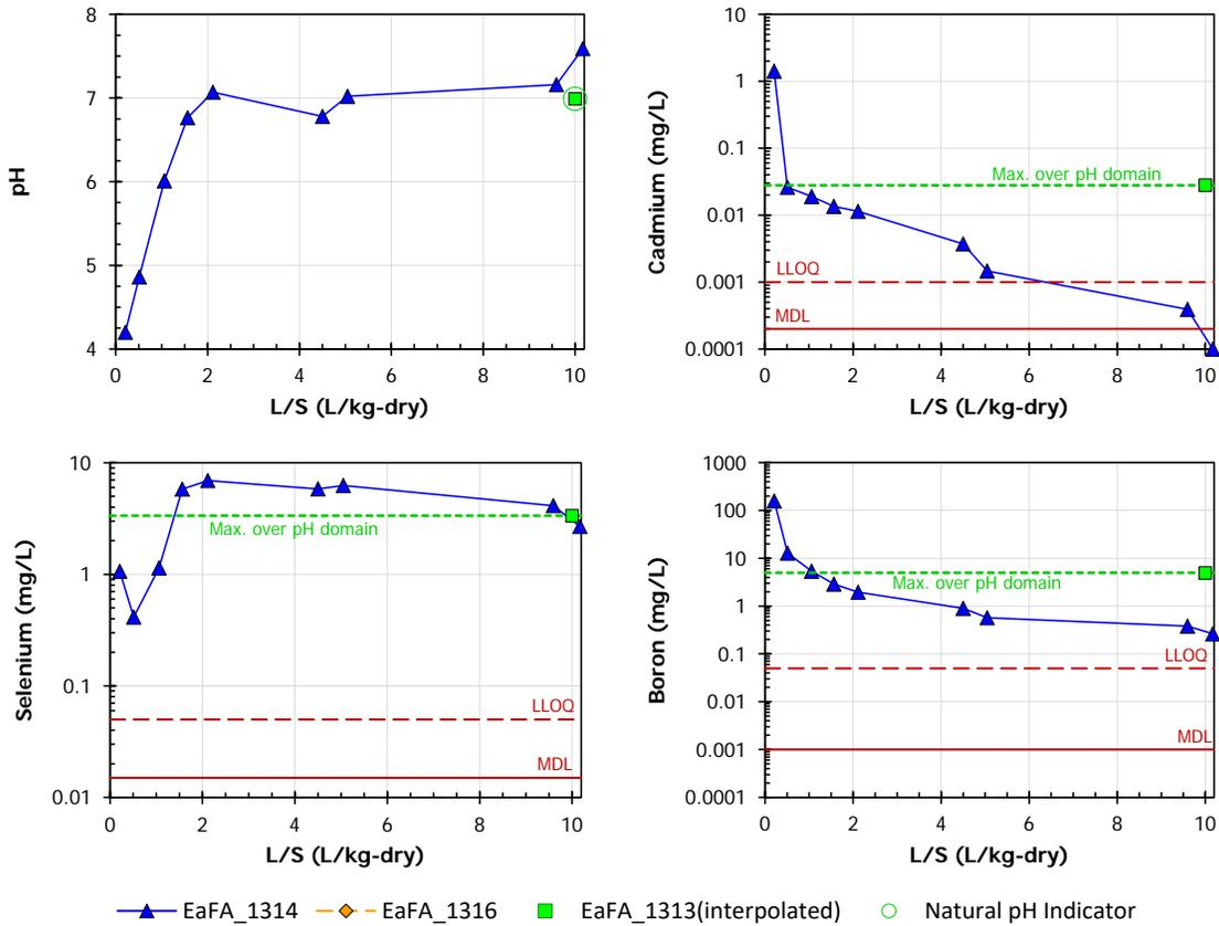
**Figure 5-1. Eluate pH and COPC concentrations as a function of pH (left) and L/S (right) for a coal combustion fly ash (EaFA) for full LSP screening assessment: Method 1313 interpolated), Method 1314, and Method 1316.**
