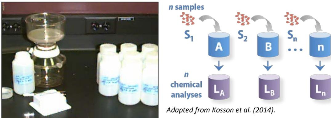
Parallel batch extractions with varying quantities of deionized water, approximating liquid-solid partitioning as a function of pH at chemical equilibrium.
