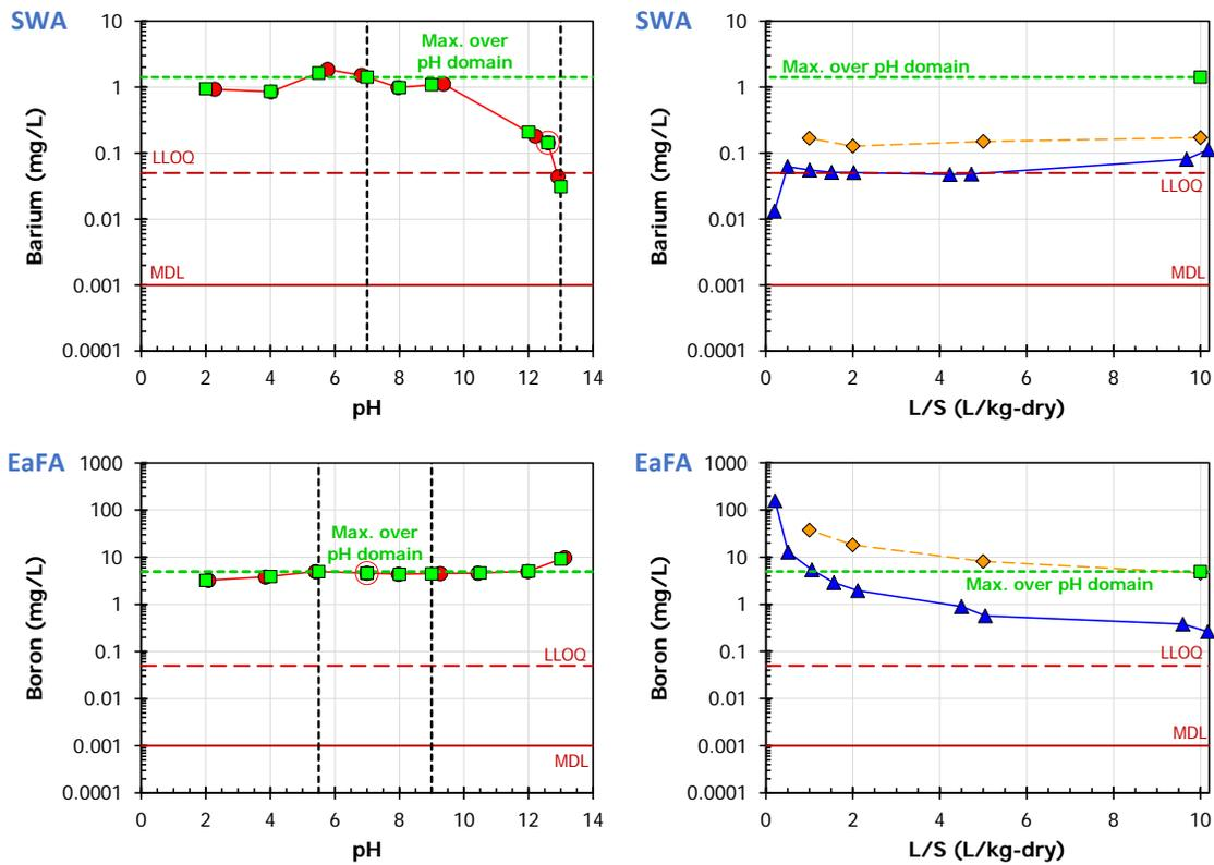
**Figure 4-5. Full LSP screening data showing examples where pH effects dominate LSP (barium in solidified waste form, SWA) and where L/S-dependence influences maximum LSP concentration (boron in coal fly ash, EaFA).**
