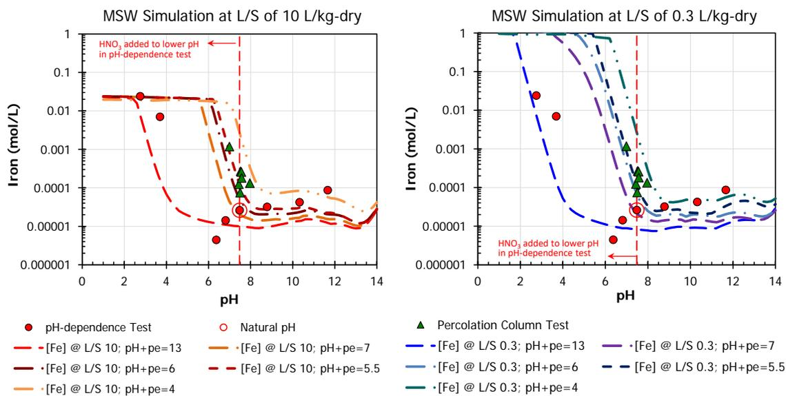
**Figure 4-7. Comparison of geochemical simulation of iron leaching at various pH/redox conditions ( $\text{pH} + \text{pE}$ ) to laboratory test results for mixed municipal solid waste (MSW) landfill material.**
