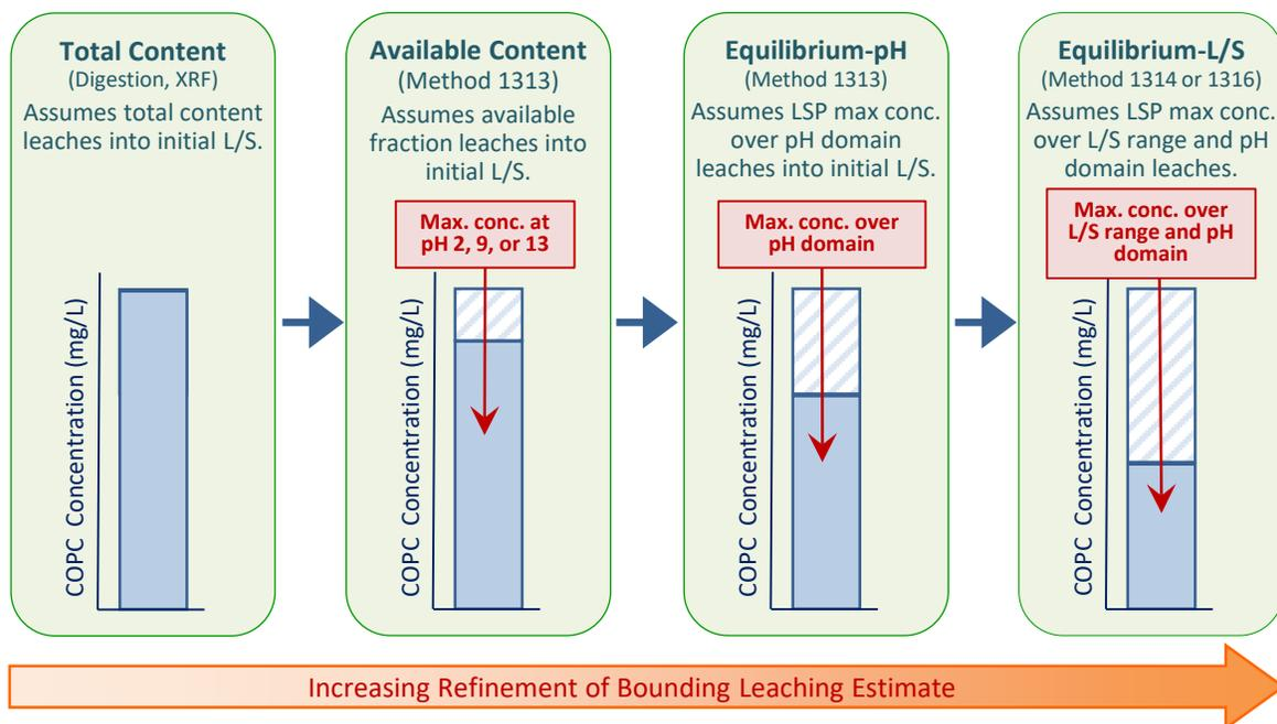
**Figure 4-2. Screening level assessments, test methods and assumed leaching conditions.**
