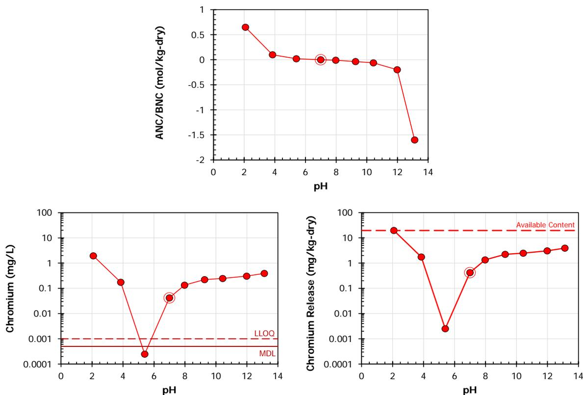
**Figure 3-2. Example results from Method 1313 for leaching from a coal combustion fly ash (EaFA):** Titration curve (top), chromium eluate concentration (lower, left) and chromium release with available content displayed (lower, right).
