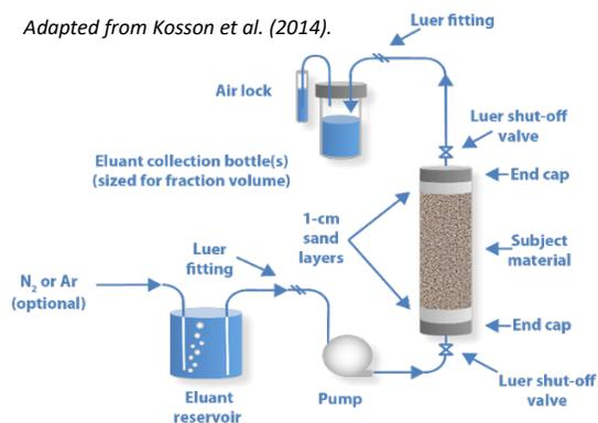
Up-flow percolation column to collect eluates at specified L/S values, estimating liquid-solid partitioning at percolation release conditions that approximate chemical equilibrium.
