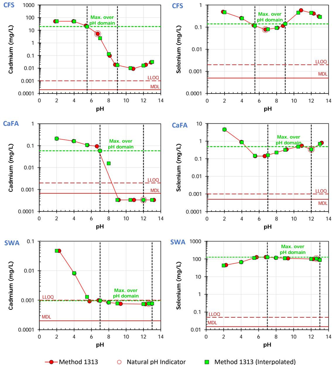
**Figure 4-3. Maximum concentration over an applicable scenario pH domain for cadmium (left) and selenium (right) from Method 1313 testing of a coal combustion fly ash (CaFA), a contaminated soils (CFS) and a solidified waste form (SWA).**
