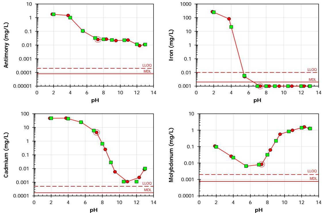
**Figure 4-12. Comparison of measured Method 1313 eluate data (red dots) for a contaminated smelter site soil (CFS) with interpolated test results (green squares) using linear interpolation of log-transformed concentration data.**
