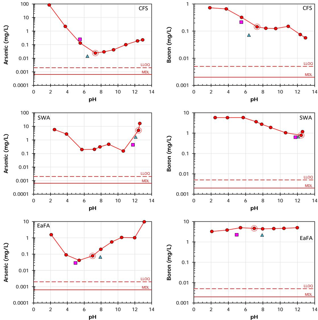
**Figure 3-9. Comparison of TCLP and SPLP results to pH-dependent leaching from Method 1313 for a contaminated smelter site soil (CFS; top), a solidified waste form (SWA; center) and a coal combustion fly ash (EaFA; bottom).**
