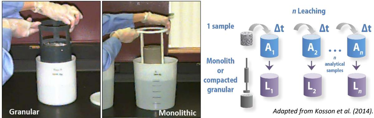
Sequential extraction of a monolith or compacted granular specimen to determine the maximum rate of release by diffusion and dissolution processes.
