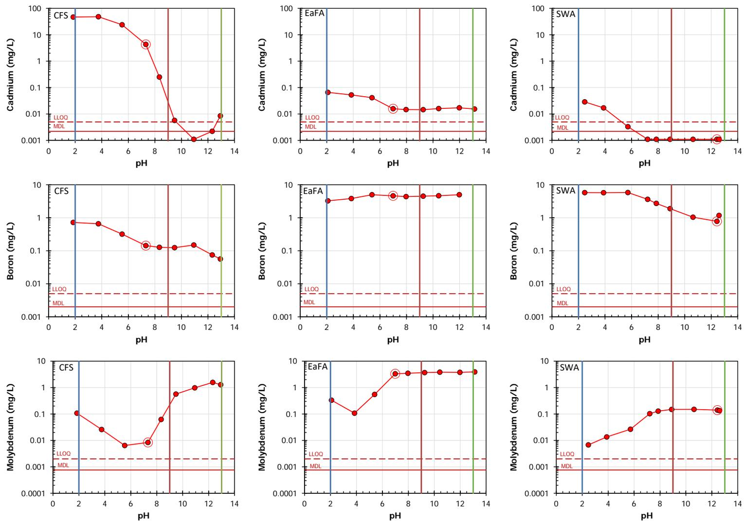
**Figure 4-11. Comparison of eluate concentrations at specified pH values of 2, 9, and 13 used to determine the available content: Contaminated smelter site soil (CFS; left), coal combustion fly ash (EaFA; middle) and solidified waste form (SWA; right).**
