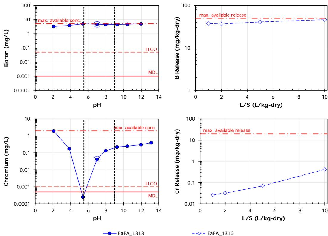
**Figure 4-17. Available content-limited leaching of boron and solubility-limited leaching of chromium from a coal combustion fly ash (EaFA) based on the results of Method 1313 (left) and Method 1316 (right).**
