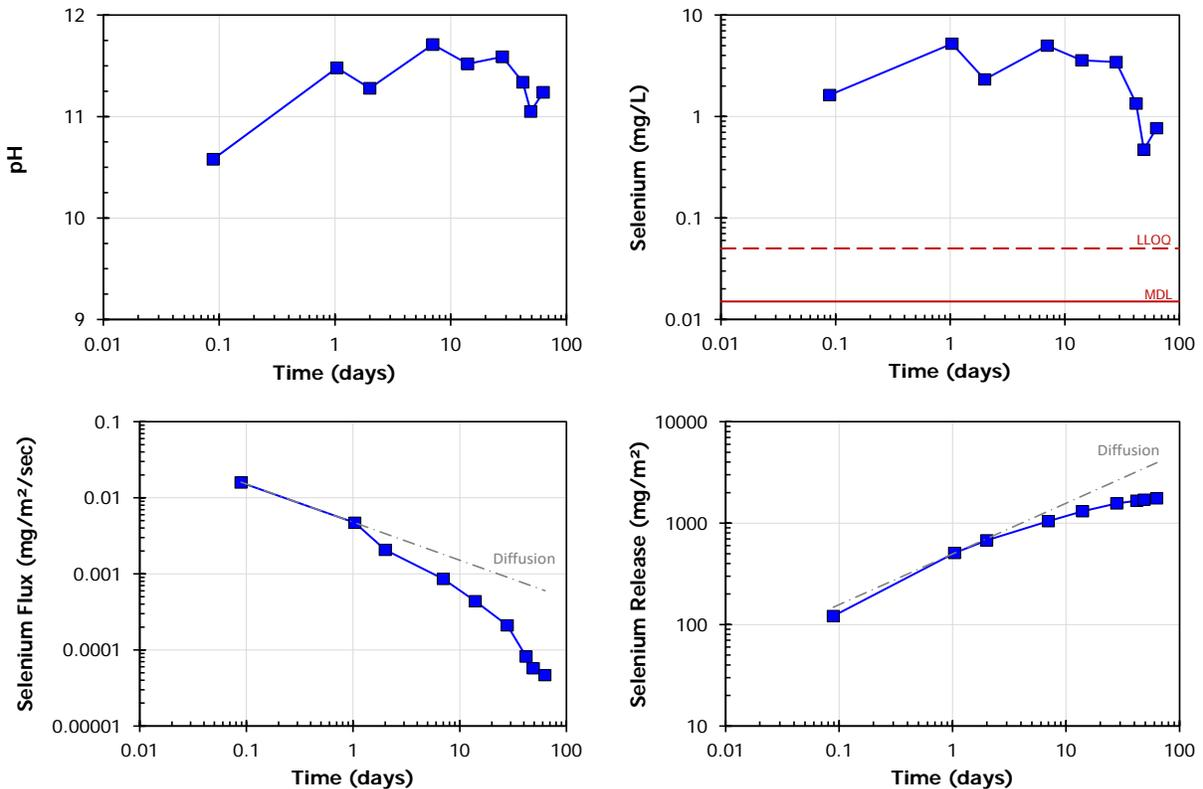
**Figure 3-6. Example results from Method 1315 for selenium shown as a function of leaching time from a solidified waste form (SWA):** Eluate pH (upper, left), eluate concentration (upper, right), mean interval flux (lower, left) and cumulative release (lower, right).
