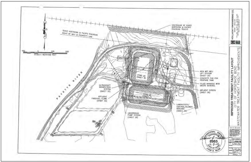
Figure A-3. Detailed layout of Horseshoe Bend WWTP.
