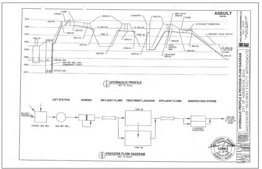
Figure A-4. Hydraulic profile and process flow diagram for Horseshoe Bend WWTP.
