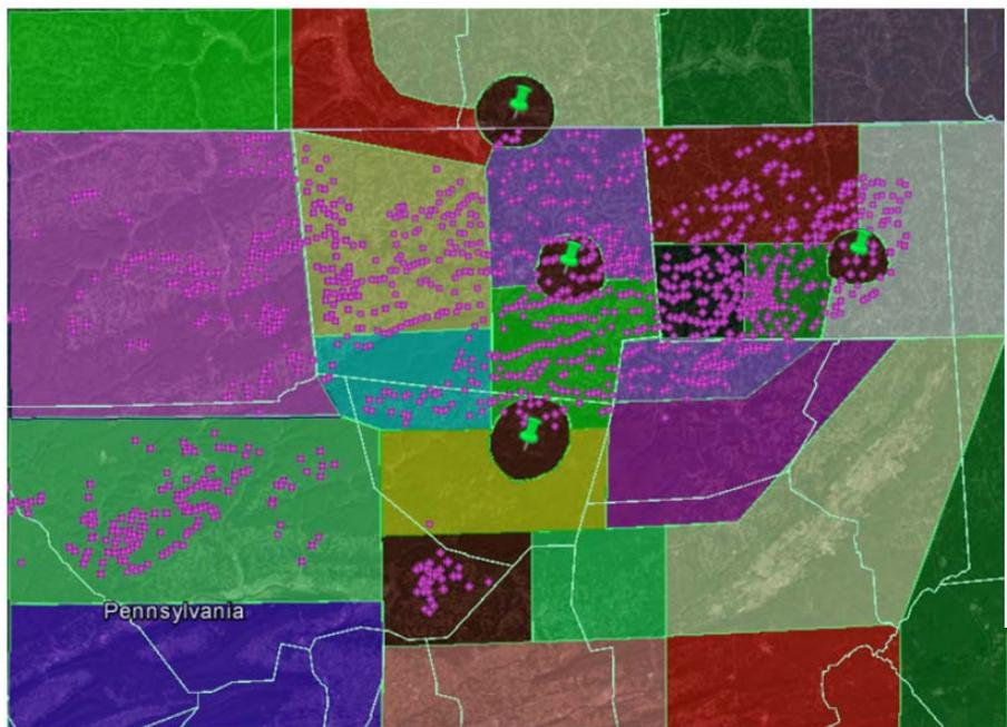
Diagram of the different flux sub-regions used in the inversion. Towers (green pins) and wells (pink dots) are plotted overtop
