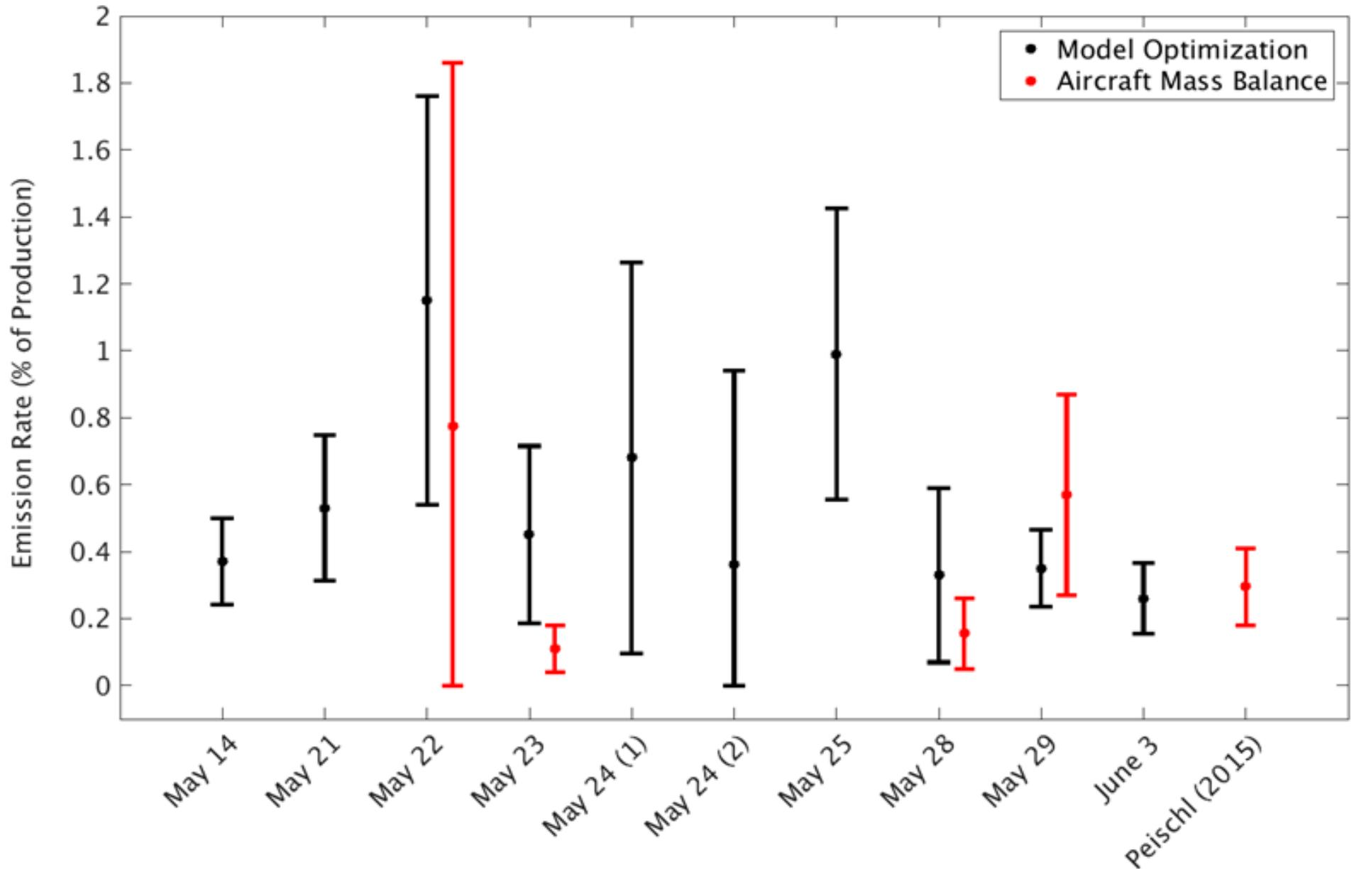
Optimal mean leakage rate based on 10 flights in May 2015: **0.39% of production**
