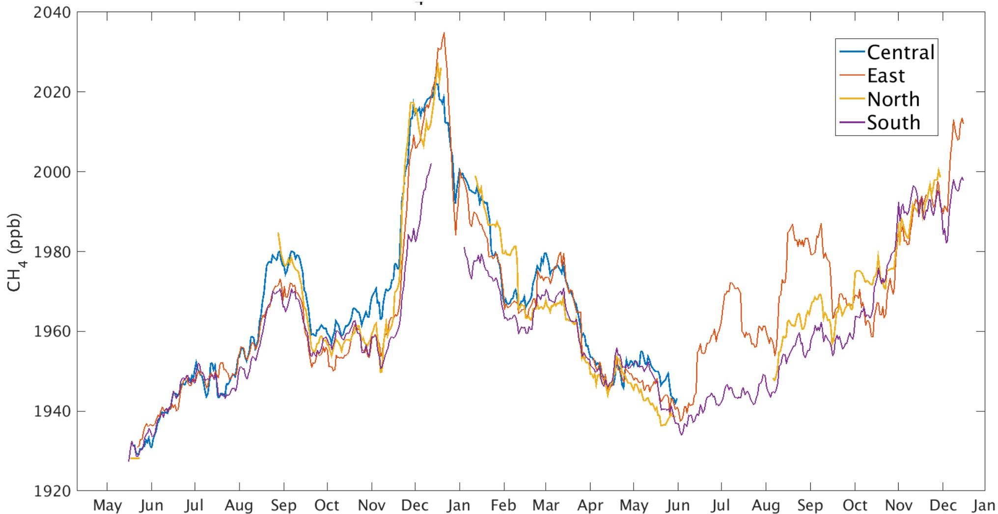
CH<sub>4</sub> mixing ratio measurements over 2015-2017 from the four CRDS CH<sub>4</sub>/<sup>13</sup>CH<sub>4</sub> instruments (in ppb)
