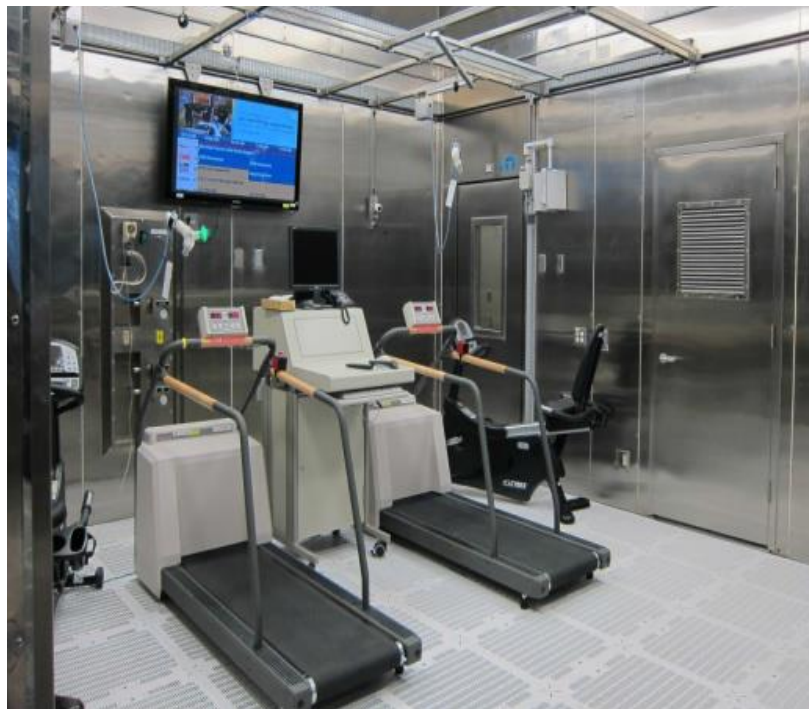
Chamber used for controlled exposure ozone studies at the University of North Carolina at Chapel Hill. (EPA OIG photo)
