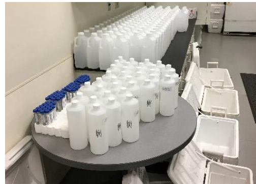
Georgia State Laboratory preparation of drinking water sample bottles to be sent to public water systems. (EPA OIG photo)
