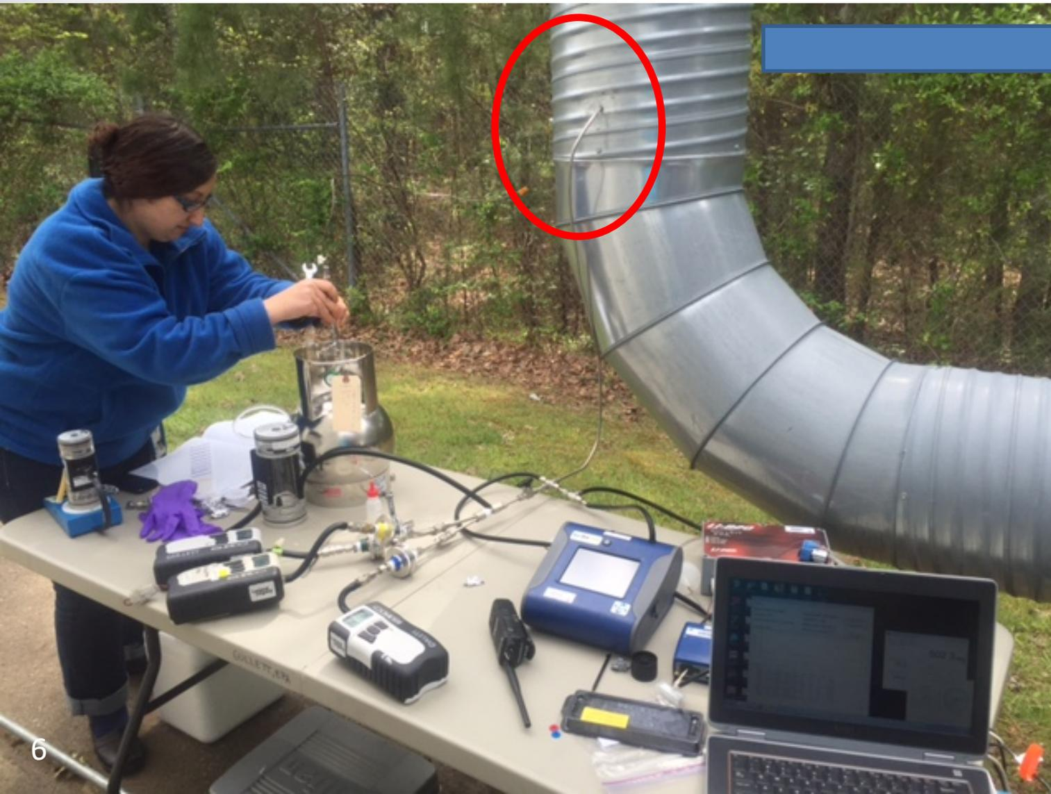
Sample emissions in the exhaust duct from the burn hut.
