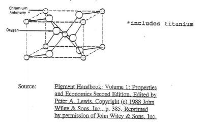
The basic chemical formula of CAT is (Ti,Cr,Sb)0<sub>2</sub>. CAT exhibits outstanding chemical, heat and light stability with extremely high resistance to light and weather. CAT remains insoluble in water, organic acids, dilute alkalies, and most inorganic acids. In order to perform the solubility study of constituent metals from CAT, the testing laboratory working on behalf of a CPMA member needed to dissolve the compound. After several attempts, the laboratory concluded:
