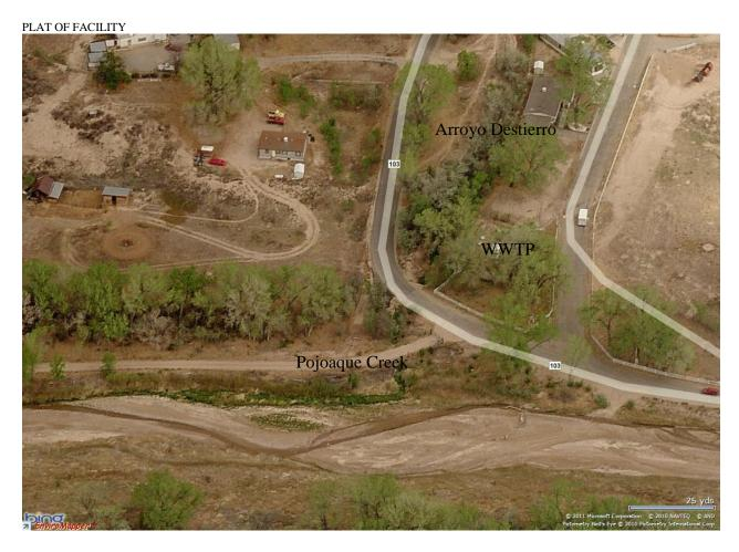
The wastewater treatment plant consists of a modified extended aeration activated sludge process with secondary clarification, chlorination (calcium hypochlorite tablet feeder) and de-chlorination (sodium sulfite tablet feeder). Sludge is wasted to a holding tank and is taken away for disposal by a contracting firm (S&R Septic). S&R Septic disposal facility is located off Tune Drive that intersects NM Hwy 65. S&R Septic operates under DP-465 issued by the NMED.
