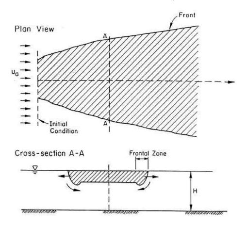
**Figure 3. Plume Buoyant Spreading**
