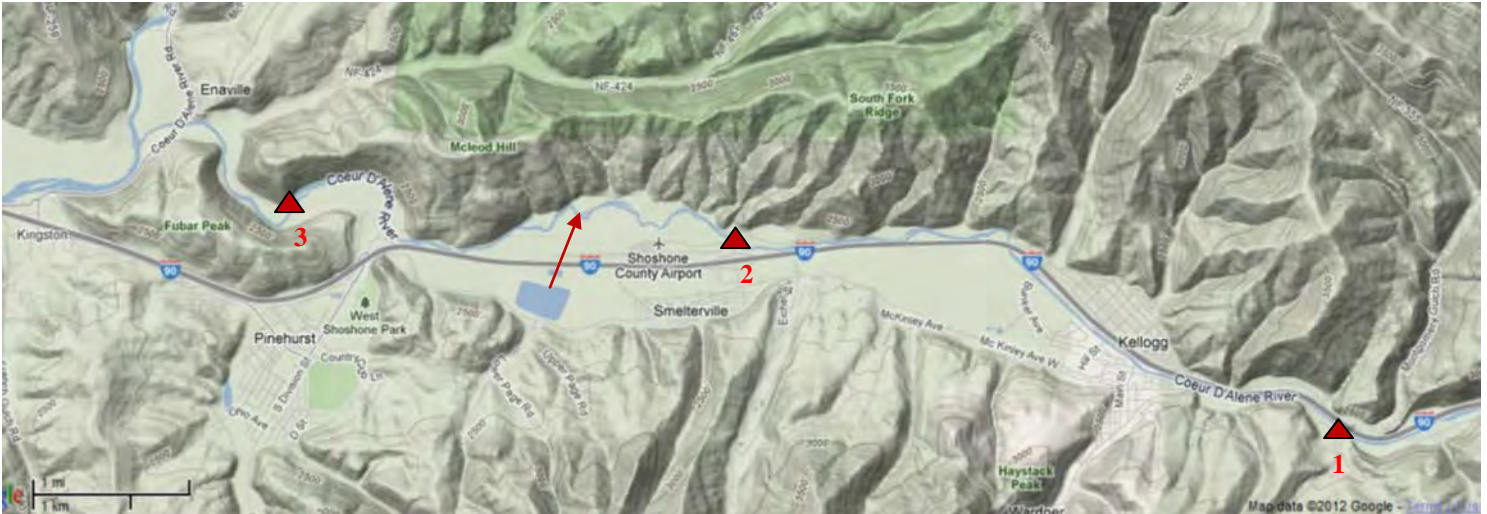
Figure 8. River Flow Monitoring Stations in the Vicinity of the Outfall
