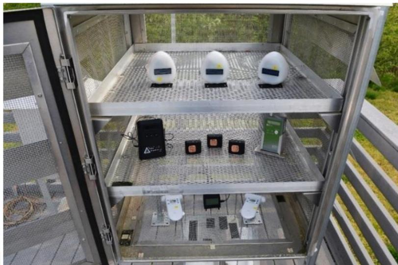
Example of sensors being tested in triplicate
