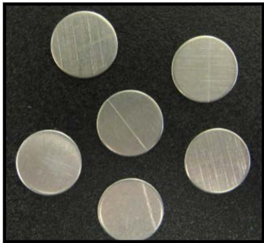
Fig. 2: Examples of typical unacceptable 430 SS carriers.
