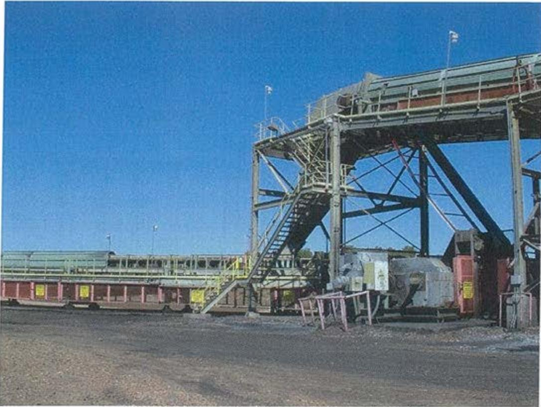
**Figure 4. Belt-to-Belt Transfer Through Chute**
