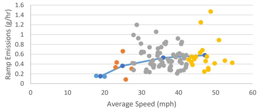
On-Ramp Brake Wear g/hr Emissions vs Average Speed
