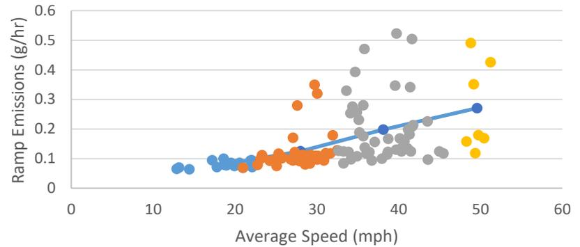
Off-Ramp Brake Wear g/hr Emissions vs Average Speed
