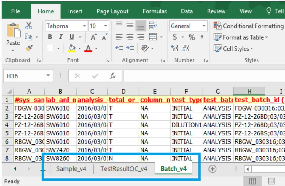
Figure 5: Excel Workbook with Sections named properly for opening all sections directly into EDP.
