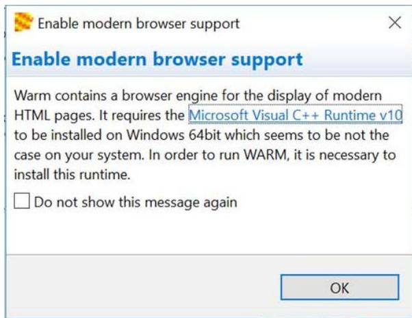
Figure 2. Message displayed if the MS Visual C++ Runtime v10 is missing
