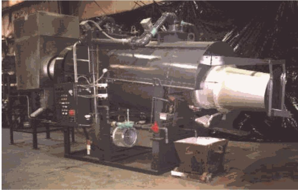
Figure 1: Photograph of Coreco Sweat Furnace and Afterburner (Models 1231 and 1848)
